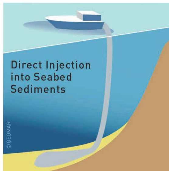
Figure 5.8 Liquid/Solid CO 2 placed into unconsolidated deep-sea sediments
